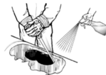
Hand Sawing Asbestos Cement Pipe
