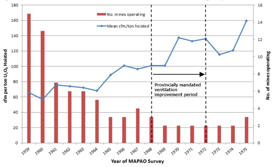
Figure 4: Ontario Uranium Mines Mean Annual Total Mine Ventilation (cfm/ton hoisted per day (thousands)
