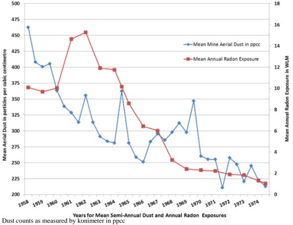
Figure 12: Semi-Annual Mean Ontario Uranium Mine Dust Counts and Radon Exposures, 1958-1975
