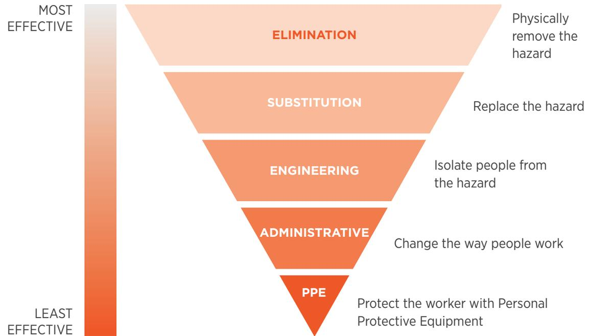
Figure 2. Hierarchy of hazard controls (24)
