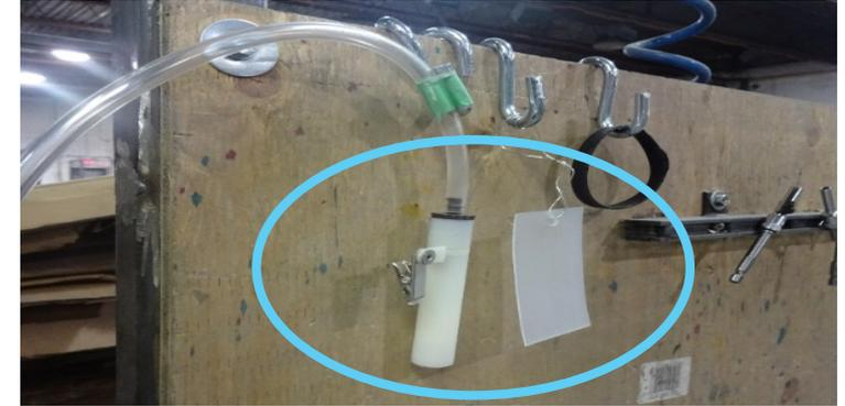
Co-deployed active and passive samplers at the workbenches and central work area.
