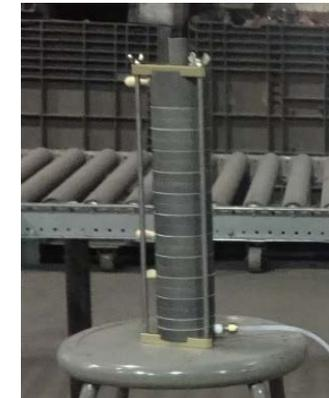
Deployed Micro-orifice Uniform Deposition Impactor (MOUDI).
