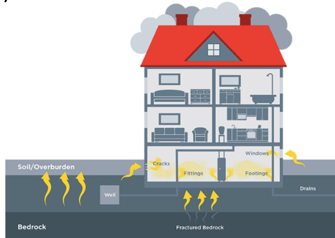
Radon is a radioactive gas that is released when uranium breaks down in the ground. It can infiltrate our homes in the various ways pictured here but mitigation strategies can reduce this exposure in both new and existing structures.
